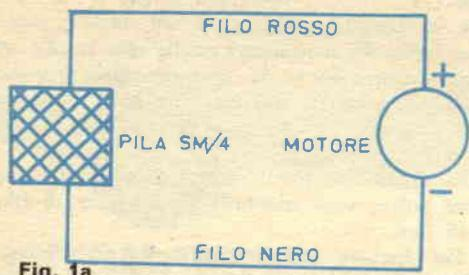
**SCHEMA ELETTRICO CON 1 PILA SM/4**
